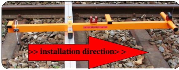
Measure the inclination with an adjustable spirit level with rotatable indicator.
