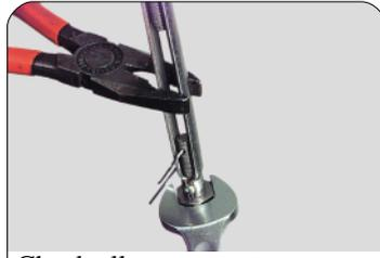
Check all counter nuts once more. Block turnbuckles with counter nuts.
