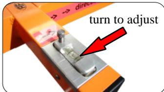
Place the JIG with red side to the installation direction. Adjust the spirit level for the red side.
