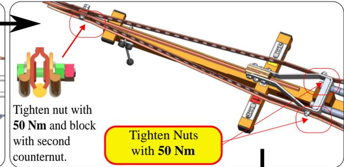
Tighten nut with 50 Nm and block with second counternut.
