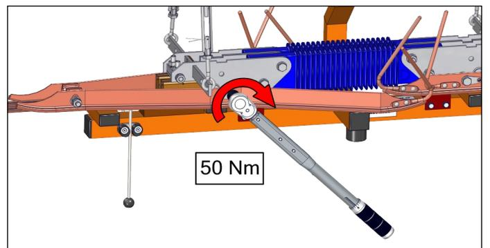
Tighten the nuts to **50 Nm** and lock them with the counter nut.
