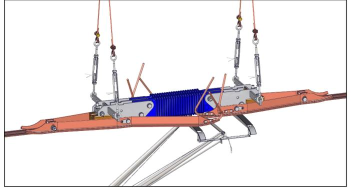
A well adjusted section insulator can be lifted with 120 N using a spring balance attached to the skid ends with arcing horns without inclining or the suspension cables becoming loose. If the suspension cables are no longer tight when raised, the section insulator must be raised gradually (by 10 mm) until the suspension cables are tight again.
