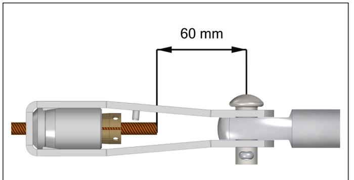
Install the messenger wire insulator and attach the saddle clamps and suspension cables to it.
