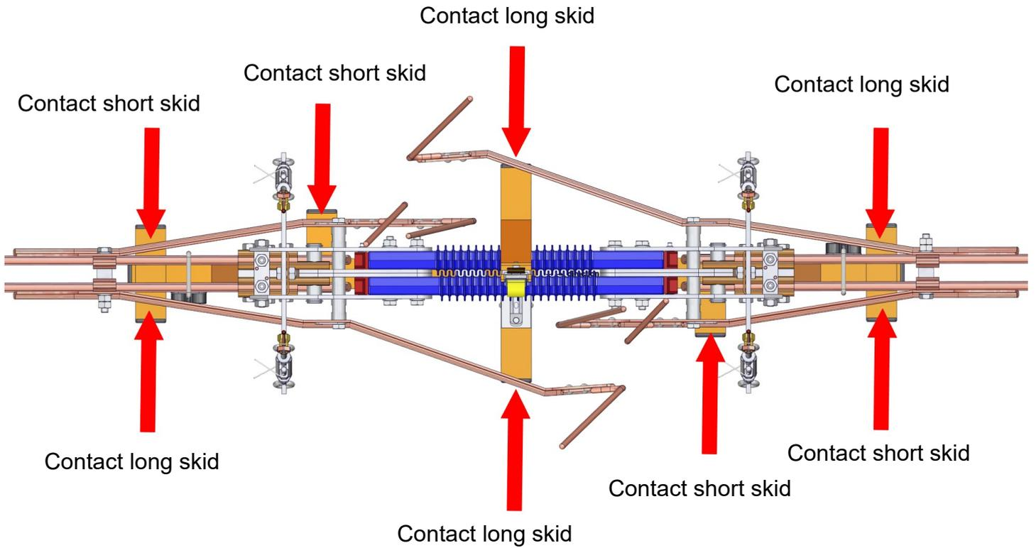
Tighten the nuts of the skids with **50 Nm**.
