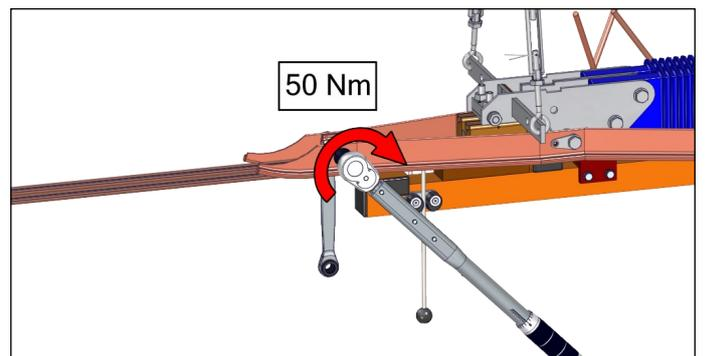
Remove the installation JIG from the insulator body.
