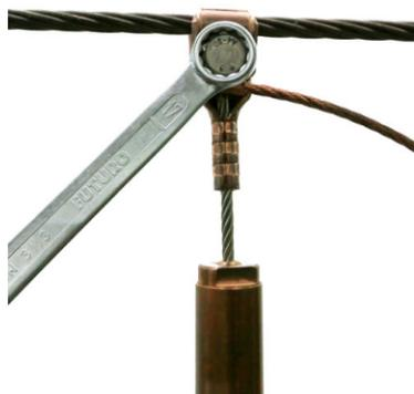
2. Install the compressed delivered cable dropper clamp at the catenary (messenger wire) cable. Tighten the bolt with a torque wrench of 25 Nm.
