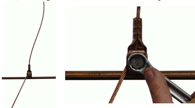
4. Definite adjustment of SHP4. Pull down the cable until you reach a measurement of 120mm (4¾ In).
